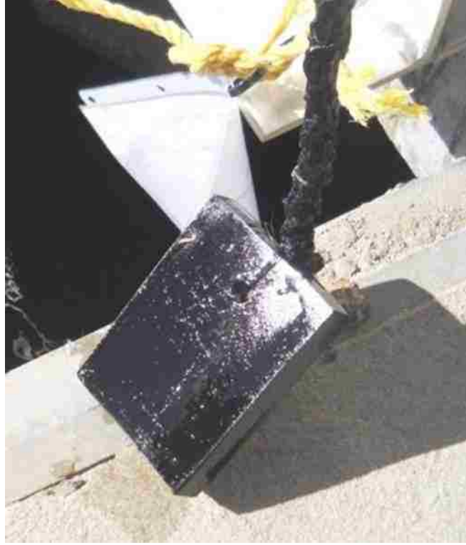
Figure 32 Slime Sample Showing Accumulation on Braided Line before Cutting and Replacing with Nylon Line
