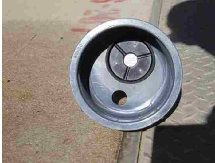
Figure 21 Bottom View of Cap with OdaLog
