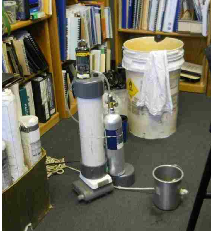
Figure 35 Office Set-Up for Dry Chamber Testing
