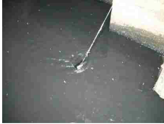
Figure 29 Sample Hanging in Effluent Channel
