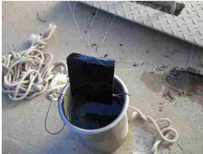
Figure 33 Slime Sample after Tying with Nylon Line - Ready for Testing
