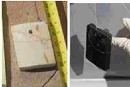
Figure 30 Sample Before and After Hanging in Flow Eight Days
